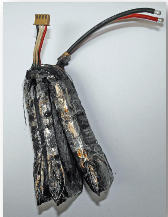
FIGURE 3. DAMAGED BATTERY PACK AFTER THE TEST
