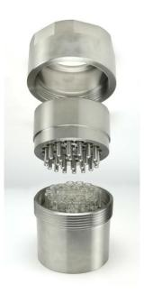
The bottom section is the vial holder on which the top plate is placed. The top plate may or may not have an integrated reflux head. On top is the clamp that fits over the top plate and screws down onto the bottom vial holder section.
