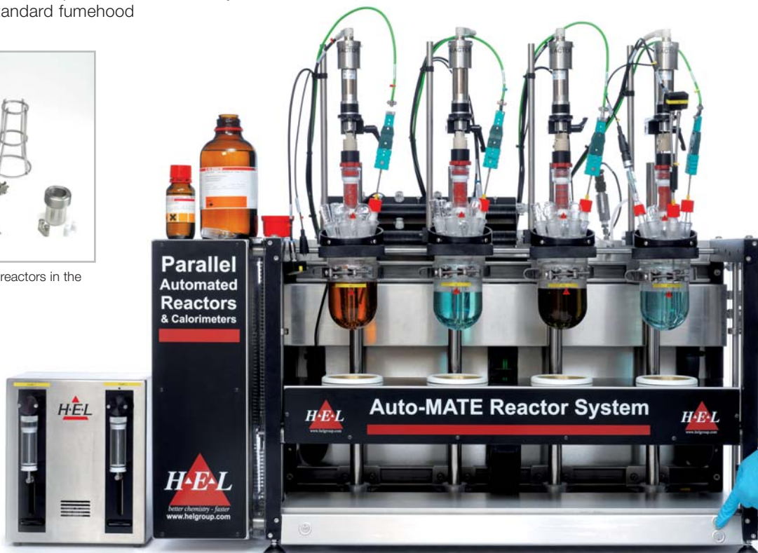
AM4 with 350ml glass vessels interchangeable with other high and low pressure reactors of different sizes. Movable jacket, independent temperature control and monitoring of each reactor
