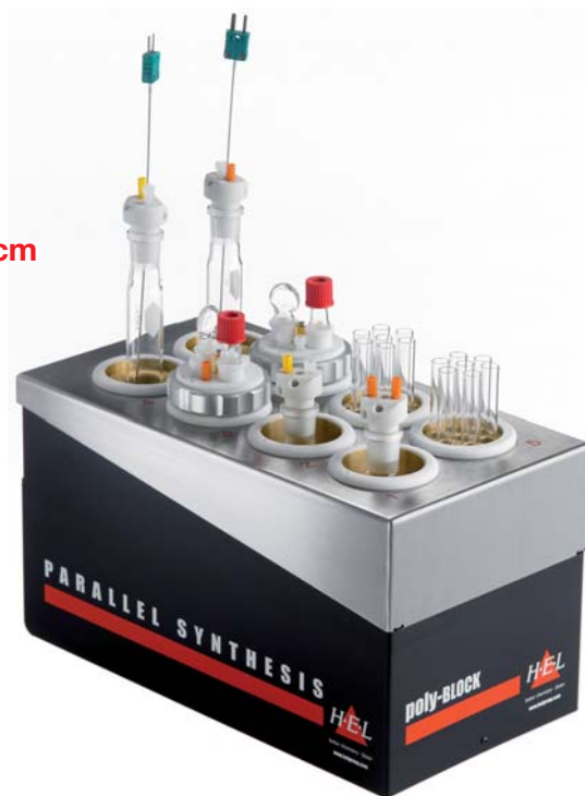
PB8 Independent temperature ramps – 30ml vessels
