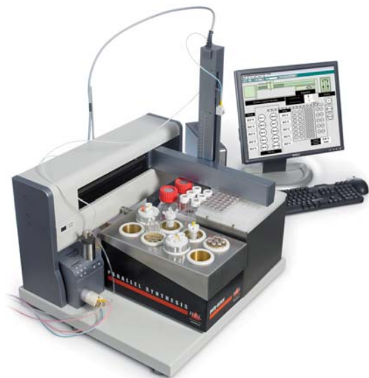
LP ChemSCAN using PolyBLOCK PB8. 2 PolyBLOCKs can be served by one robot
