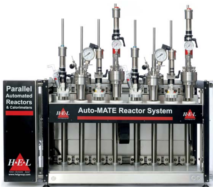
AM4 with 350ml glass vessels interchangeable with other high and low pressure reactors of different sizes. Movable jacket, independent temperature control and monitoring of each reactor
