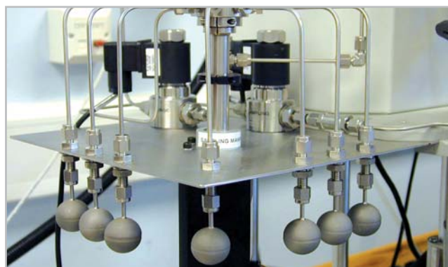
Fully automated high pressure sampling. Separate system available for low pressure applications
