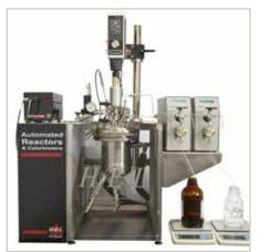
Metal alloy reactors rated to 100 bar/350 °C, with common cover plate up to 20 L. Floor standing or bench scale according to size.
