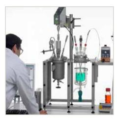
Metal and glass vessels on common stand to allow easy switching of applications with shared software and electronics.
