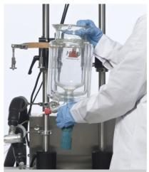
Vessel pulls out by undoing just one support clamp
