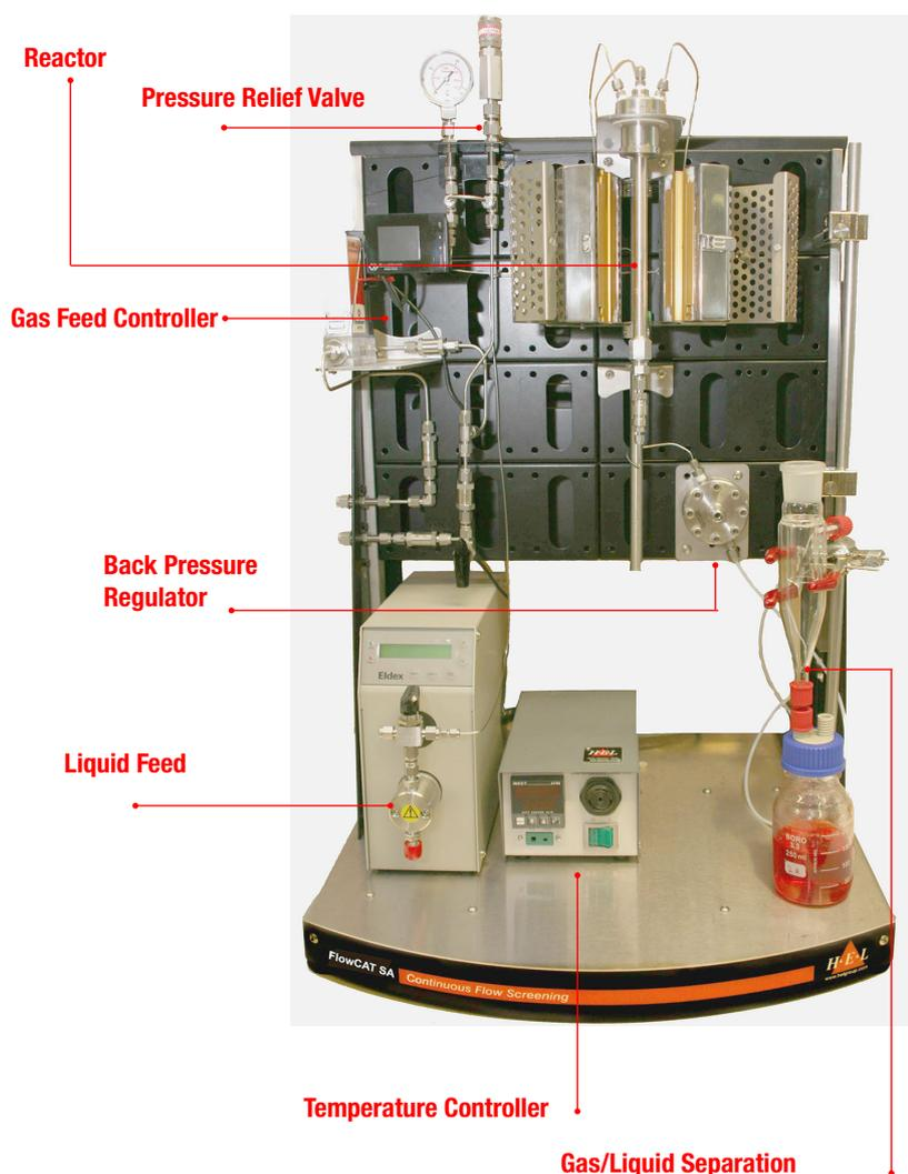
The HEL FlowCAT SA is a low cost, high performance reactor for continuous flow heterogeneous catalysis for use in applications including hydrogenation, carbonylation, oxidation and is widely used in the pharmaceutical and fine chemical industries.
