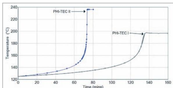
Effect of  $\phi$ -factor (thermal inertia) on runaway reaction
