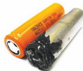
AA Batteries after a test in a 'Standard' Phi-TEC BTC
