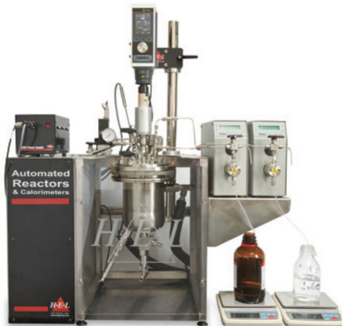
1 L high pressure reaction calorimeter
