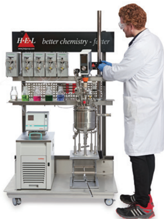
2 L pressure reactors with complex feeds and sub-ambient temperatures
