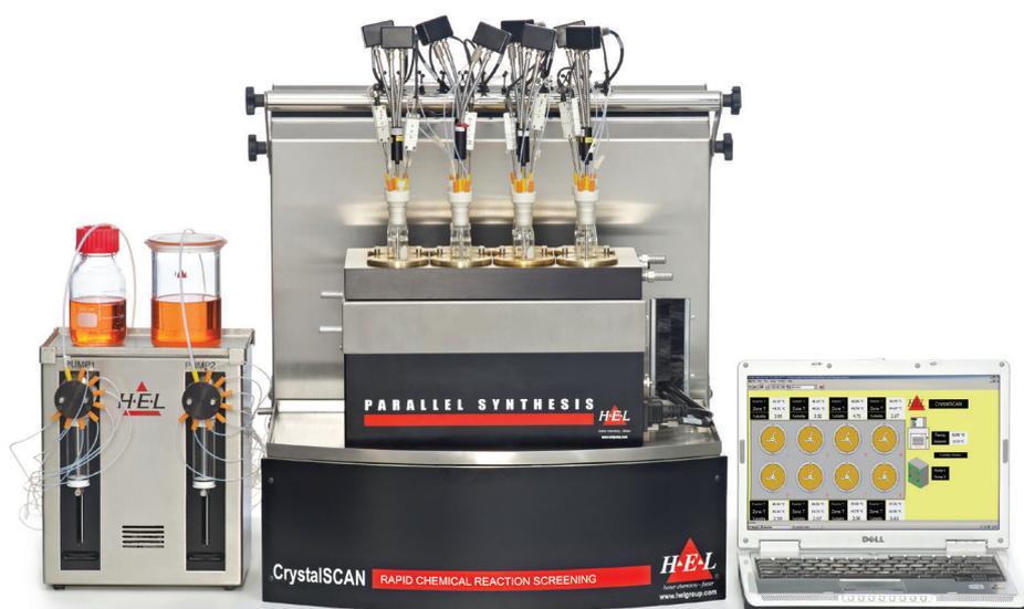
CrystalSCAN system with 8 reaction zones
