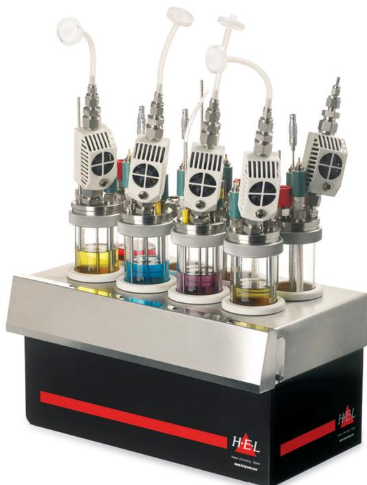
PolyBLOCK 8 parallel automated reactor system
