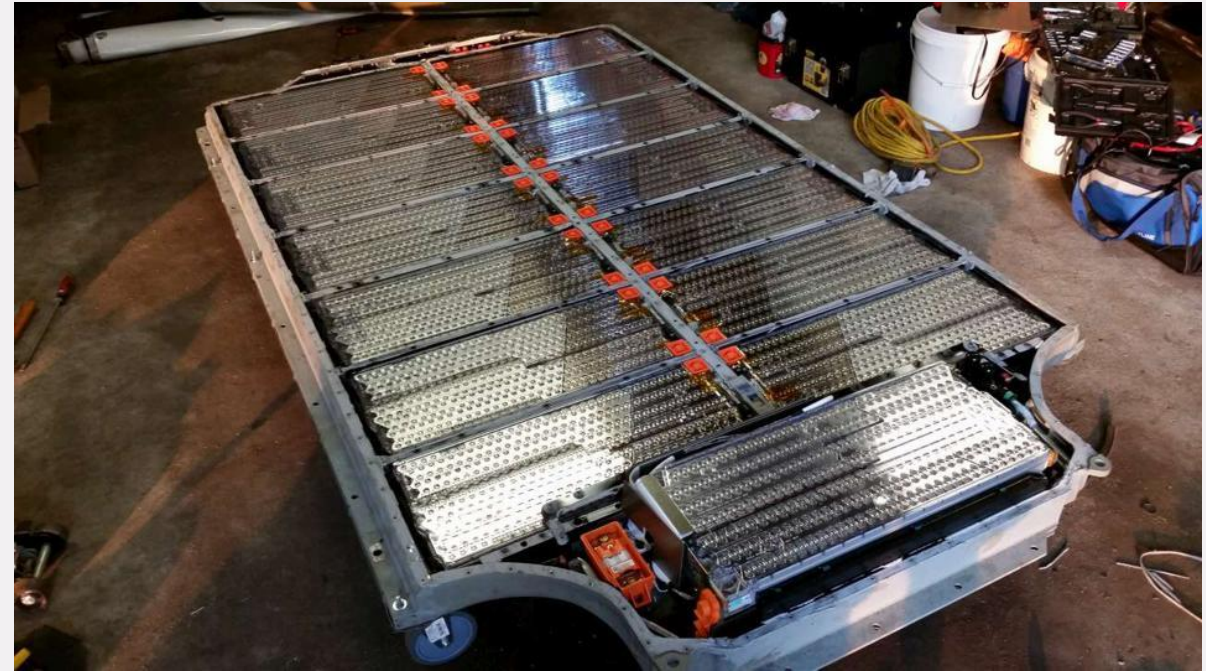
Tesla Model S standard 100kWh battery pack – All rights go to https://www.forbes.com/sites/arielcohen/2020/12/30/teslas-new-lithium-ion-patent-brings-company-closer-to-promised-1-million-mile-battery/?sh=3b8c012633e3
