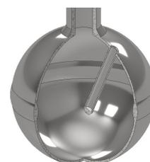
Fig 3. Cross-section of spherical test cell, showing thermowell
