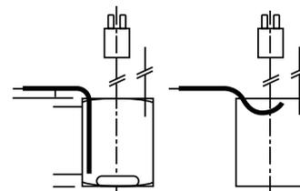
Fig 5. Long feed line (left) and swan neck feed line (right)
