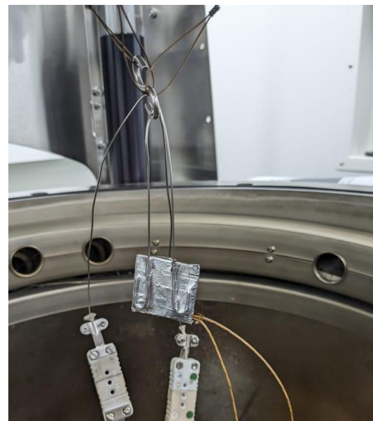
Figure 2. Battery suspended from the lid of a BTC-500 using an S-hook. The battery was covered with foil to ensure a thorough heat distribution from the heater. At the bottom, the thermocouples used for temperature tracking can be seen connected to the battery.
